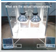
O Compared with uncoated glass, temperature difference was 15.5 °C !!
